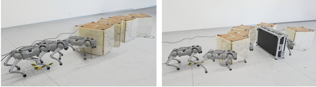
Figure 7: Snapshots from the hardware deployment for the single object and single wall tasks. The mass of the box is 5.5 kilograms with a dimension of (0.55, 0.55, 0.5) meters.
